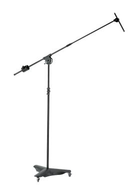
Mobile heavy steel microphone stand for studio or stage. 10 kg cast metal base, low centre of gravity for high level safety with 3 lockable castor wheels. Rod combination extends to over 2 m with additional locking mechanism. Extendable boom arm with a 3 kg counterweight and 5/8" connecting thread. Additional mini boom arm with 5/8"- and 3/8"- connecting thread, fully adjustable regardless of the position of the main boom arm, e.g. to use with studio microphones.
